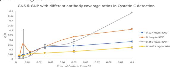
**Figure 2** Detection of Cys C from 0.003125 mg/L to 0.1 mg/L with GNS conjugated antibody's concentrations as 0.167 mg/ml and 0.1 mg/ml; GNP conjugated antibody's concentrations as 0.441 mg/ml and 0.11025 mg/ml.
