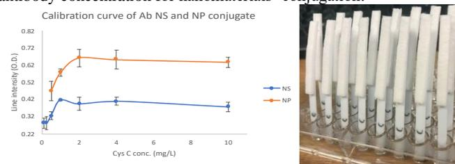
**Figure 3** Left) Detection calibration curve of Cys C from 0 to 10 mg/L; Right) Half-moon signal suggests strong binding between paired antibodies, together with undistinguishable signals between higher Cys C conc.
