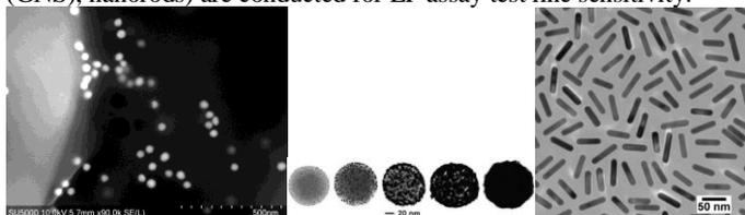
**Figure 1** Left) 40 nm gold nanoparticles under SEM; Middle) 150 nm gold nanoshells (Oldenburg, 2019); Right) 55 nm x 15 nm gold nanorods (Joshi, Yoon, Hardin, Emelianov, & Sokolov, 2013).
