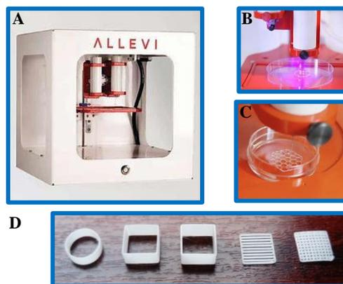
**Figure 1** Images of Allevi 3D-printer with melt extrusion capability (A-C). A range of initial 3D-scaffolds of PCL hard tissue, from left to right, 10 mm cylinder, 10 mm cube, 10 mm cube (repeat), 10 mm cube with inset geometry of lines and 10 mm cube with inset geometry of a grid (D).
