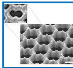
**Figure 2** Scanning electron microscopy image of 'accordion-like honeycombs' with anisotropic structure for cardiac tissue engineering, created by Engelmayer *et al.* [5].
