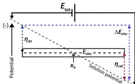
**Figure 1** Schematic representation of electric field and overpotential positions on a bipolar electrode placed between two appropriate driving electrodes.
